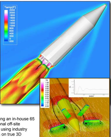
TGV performs complex aerodynamic analysis using an in-house 65 GigaFLOP super computer with access to additional off-site computing resources. Simulations are performed using industry standard NASA USM3D and FUN3D flow solvers on true 3D meshes.
